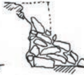
3) WITH RAINFALL, THE WALL COLLAPSES
